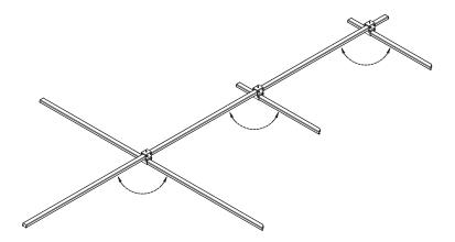
VARIABLE crossovers provide the mechanical connection for building variable angles. The VARIABLE crossover rotates to connect one single-deck length of busSTRUT to another single-deck length at any angle. Necessary rotation can be made in the field.
