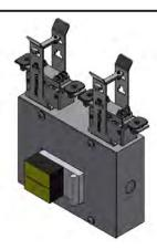
CUBEFused line-feed (up to 40 Amps) can be positioned anywhere on busSTRUT to reduce the length of homeruns. Features a pair of 3 Pole Fitters that power up to two 40A circuits; 80A max. Available in galvanized, powder coated white and black. Universal 120/277V. Mounts to both single and double-deck busSTRUT/40. Factory installed Fuse Holders.
