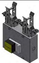
CUBEFused line-feed (up to 20 Amps) can be positioned anywhere on busSTRUT to reduce the length of homeruns. Features a 3 Pole Fitter that powers up to two 20A circuits; 40A max. Available in galvanized, powder coated white and black. Universal 120/277V. Mounts to both single and double-deck busSTRUT/20. Factory installed Fuse Holders.
