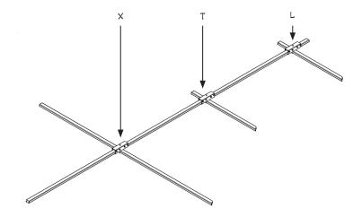
Crossovers provide the mechanical connection for building runs, rows, and grids. One universal crossover serves as an X,T, or an L intercept. The ONE over ONE crossover is used when one single-deck length of busSTRUT intersects another single-deck length of busSTRUT.
