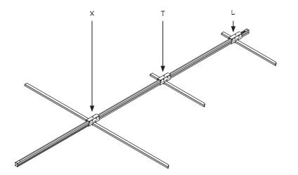
Crossovers provide the mechanical connection for building runs, rows, and grids. One universal crossover serves as an X, T, or an L intercept. The TWO over ONE crossover is used when one double-deck length of busSTRUT intersects a single-deck length of busSTRUT.
