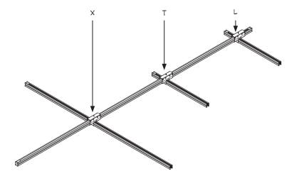
Crossovers provide the mechanical connection for building runs, rows, and grids. One universal crossover serves as an X,T, or an L intercept. The TWO over TWO crossover is used when one double-deck length of busSTRUT intersects another double-deck length of busSTRUT.
